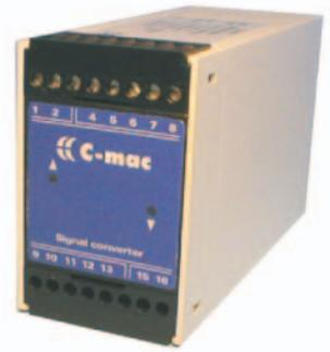
The C-mac<sup>®</sup> converter, type LR10 is used for speed monitoring, where the input signal comes from a contact, a proximity sensor, a flow transducer or similar. The unit is supplied with a 24 VDC, max. 25 mA output, which can be used to supply an external proximity sensor.
