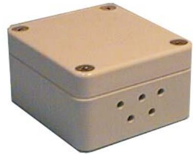
The C-mac<sup>®</sup> combined humidity and temperature sensor HS16 consists of 2 independent loop-powered circuits for monitoring of relative humidity and temperature, respectively. HS16 is available in 2 versions either with internal sensors or with an immersion tube, which is useful, if f.inst. you want to monitor the humidity and temperature in ventilation channels.
