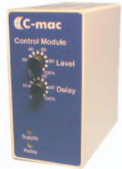
C-mac® current monitoring relay, type RC10, and voltage monitoring relay, type RV10, are universal metering relays, each supplied with 4 metering ranges, from 0,4 mA to 6 A or 40 mV to 600 V AC or DC, respectively.
