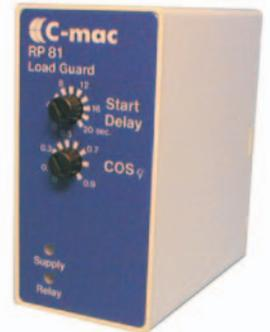
C-mac<sup>®</sup> module type RP81 is used for load monitoring of 3-phase motors, as the phase angle ( $\cos \varphi$ ) between motor current and -voltage changes in proportion to the mechanical load of the motor.
