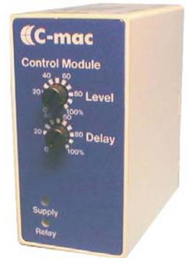
C-mac<sup>®</sup> monitoring relay, type RM34, is used for temperature metering in conjunction with Pt100 temperature sensors according to DIN 43760. A 3-wire metering principle is used, which means that the module compensates for the external cable resistance. The cable monitoring circuit also ensures that the relay will release in case of short-circuit or cable breakage.
