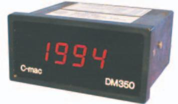
DM350 is a universal 3½-digit panel instrument with analogue inputs. The instrument has an adjustable display range between -1999 og +1999. The instrument can be used in connection with all C-mac<sup>®</sup> converters and relays with analogue outputs.
