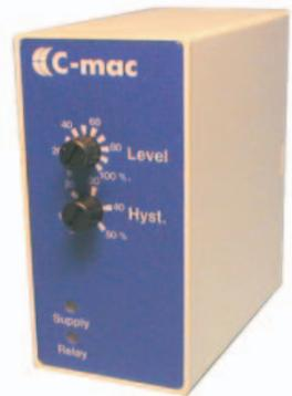
C-mac<sup>®</sup> current monitoring relay, type RC12, and voltage monitoring relay, type RV12, are universal metering relays, each supplied with 3 metering ranges, from 4 mA to 6 A or 400 mV to 600 V AC or DC, respectively.
