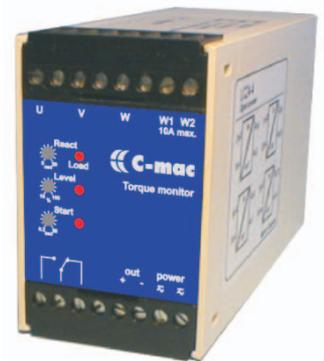
C-mac<sup>®</sup> torque monitor type MP92 is used for monitoring of the engine torque on 3-phase motors.
