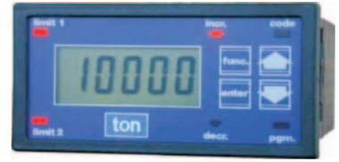
The DP545 is a 4½ digit user programmable panel instrument with backlight LCD. The instrument is supplied with universal metering inputs for direct connection to RTD and various TC temperature sensors, as well as linear current, voltage and resistance/potentiometer signals. At temperature metering, the units are programmable in °C, °F or °K.
