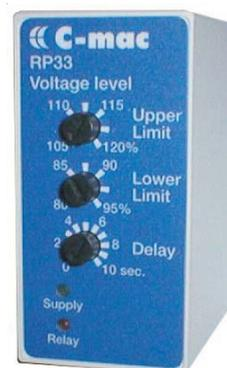
The C-mac<sup>®</sup> module type RP33 meters its own 3-phase supply voltage, and checks that all 3 phase-neutral voltages are within the adjusted limits, and in that case, the output relay is activated.
